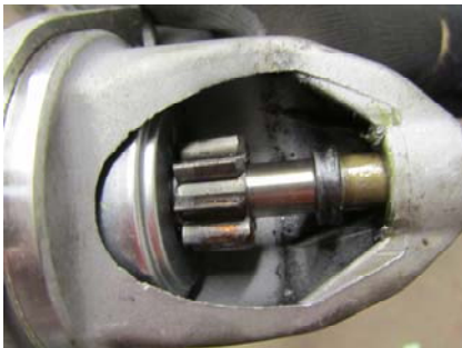
Red / blue burn marks around pinion teeth
