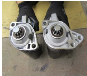
The bracket on the starter on the left has been ground off to fit – the unit on the right is how it should look!
