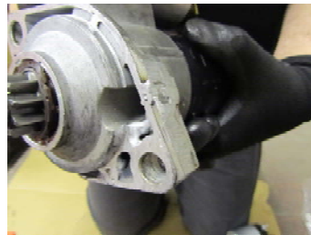
The bracket on the starter on the left has been ground off to fit – the unit on the right is how it should look!
