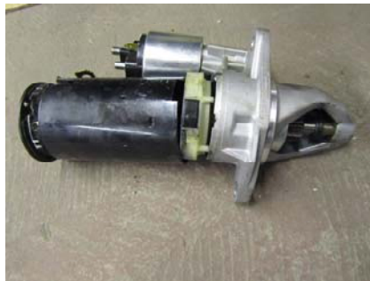
Unit held in mesh, causing collapse of brushes, brush box and armature coils
