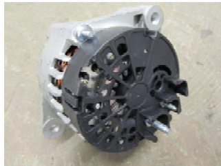
This unit was dropped by a customer, damaging the plastic cap and rectifier
