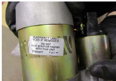
The label from a Eurolec unit was removed and placed on this non-Eurolec unit.
