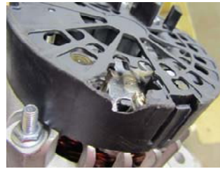
This unit was dropped by a customer, damaging the plastic cap and rectifier
