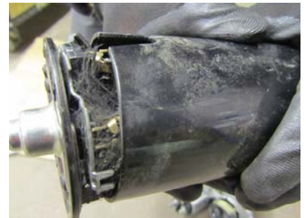
Unit held in mesh, causing collapse of brushes, brush box and armature coils
